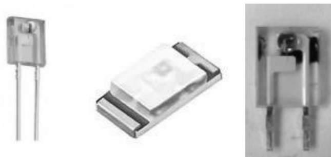
Figure 8: Components that construct the finger probe. IR LED, red LED and phototransistor, respectively.
